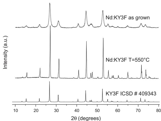
Fig. 1. X-ray diffraction pattern for Nd:KY3F synthesized nanopowder before (as grown) and after thermal treatment ( $T=550$  °C). Lowest diffractogram was obtained for a bulk crystal (KY3F) for comparison.
