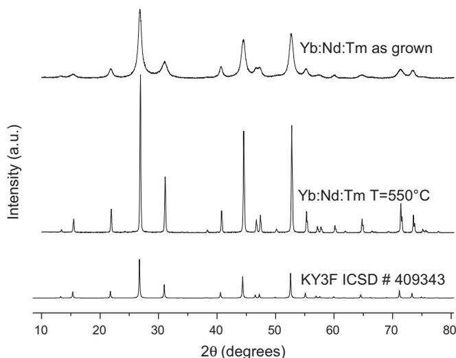
Fig. 2. X-ray diffraction pattern of Yb:Nd:Tm:KY3F synthesized nanopowder before (as grown) and after thermal treatment ( $T=550$  °C). Lowest diffractogram was obtained for a bulk crystal (KY3F) for comparison.
