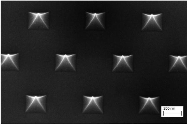
Fig. 1. Scanning electron microscope (SEM) image of several molybdenum tips with the base size of 250 nm, arranged on the hexagonal grid with the period of 640 nm.
