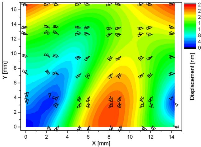
Fig. 2. Color map of the displacements of the registration marker from expected positions as measured on a demonstrator chip with 20 FEA arrays by means of e-beam lithography tool. The arrows indicate the direction of the marker displacement. Compensation for these distortions had to be done during the overlay exposures of the aperture patterns of the gate electrodes.
