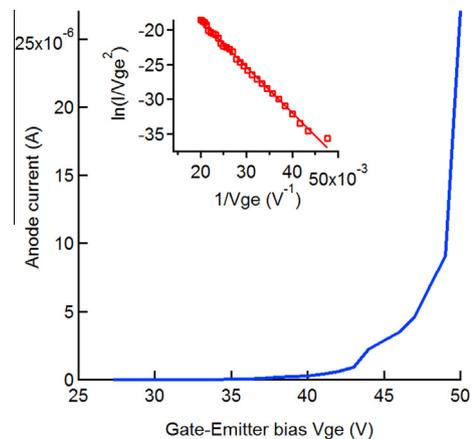
Fig. 4. Emission current vs. gate voltage characteristics of a single gate submicron-pitch FEA with diameter of 560 μm, operated in the DC mode, recorded after several days of operation. The inset shows the corresponding Fowler-Nordheim plot.
