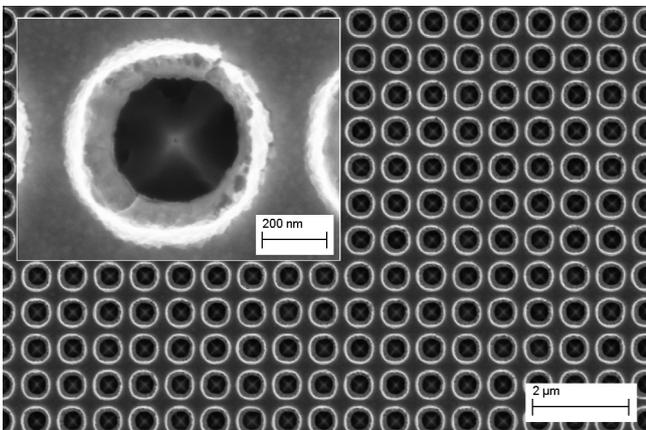
Fig. 3. A part of a 560 μm large single gate FEA with the tip distance of 750 nm and the overlay precision at any location of arrays better than 40 nm. The inset shows more detailed an individual field emitter.
