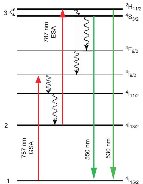
**Fig. 1.** Partial energy level diagram of  $\text{Er}^{3+}$  ions. The upward (red) arrows represent laser excitation at 787 nm. The downward solid (green) arrows represent green luminescence emission. Wavy lines represent fast nonradiative decays. GSA: Ground State Absorption; ESA: Excited State Absorption from  $^4\text{I}_{13/2}$  level. (For interpretation of the references to color in this figure caption, the reader is referred to the web version of this paper.)
