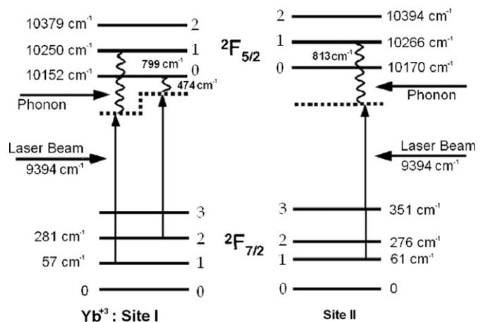
Fig. 2. Crystal-field energy diagram at  $10 \text{ K}$  for the two sites  $\text{Yb}^{3+}$  ions in  $\text{NdVO}_4$ .
