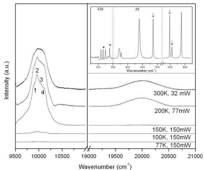
Fig. 1. Infrared and cooperative emission spectra in  $\text{Yb}_{0.1}\text{Nd}_{0.9}\text{VO}_4$  as a function of temperature. Pump ( $9394 \text{ cm}^{-1}$ ) intensity is adjusted to maximize the cooperative emission when present (see text for description of peaks 1–4). Inset: Raman active phonons of  $\text{Yb}_{0.1}\text{Nd}_{0.9}\text{VO}_4$  ( $\downarrow$ ) contributing to the  $\text{Yb}^{3+}$  excitation at  $10 \text{ K}$ . \* indicates plasma lines.
