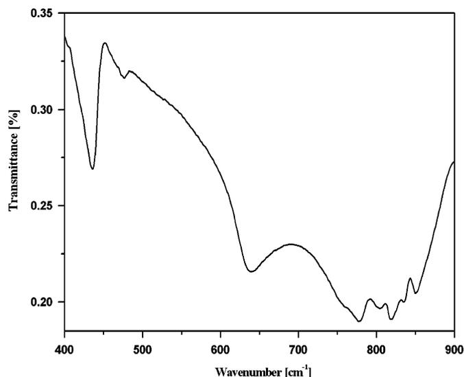
Fig. 1. IR spectrum of  $\text{KZnLa}(\text{VO}_4)_2$  in the KBr pellet at room temperature.
