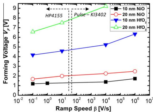
Fig. 3. Ramp speed dependent evolution of forming voltages. Measurements were performed by using either quasi-static (SPA) or pulse modes to reach a large range of ramp speeds.
