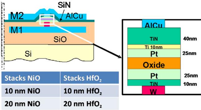
Fig. 1. Schematic of the capacitor-like resistive memory structures. The test devices are in simple 1R configuration (i.e. no series selector fabricated next to the device).
