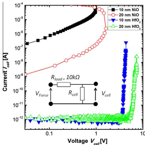
Fig. 2. Forming operation measured in quasi-static mode with a HP 4155 SPA on HfO<sub>2</sub> and NiO-based memory devices. Typical  $I$ - $V$  characteristics measured under a voltage ramp force of 0.1 V/s (each characteristic is the average of 20 devices).
