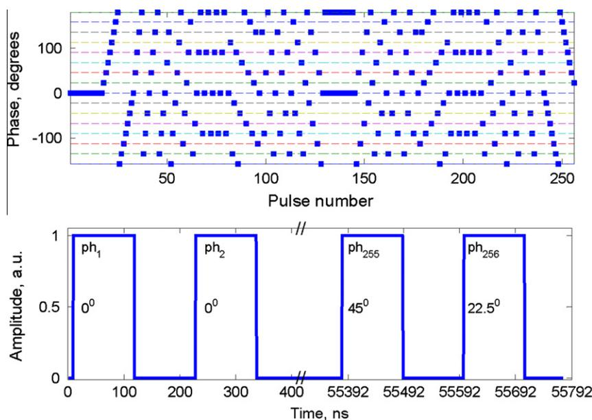
**Fig. 1.** The pulse sequence that was used to produce the spectra in Fig. 2 consisted of 256 pulses of 109 ns with the 16 different phases selected as shown in part a. The time required for the complete sequence was about  $56 \mu\text{s}$ . The detailed timing of the first 2 and last 2 pulses is shown in part b. Data were acquired continuously at 4 ns intervals during the entire pulse sequence, but only the signal corresponding to times between the pulses was analyzed.
