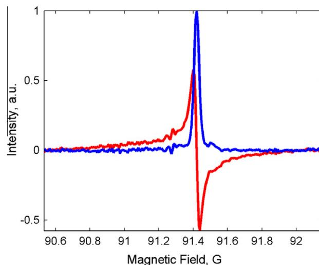
**Fig. 2.** EPR spectrum of the trityl radical obtained by means of Frank sequence EPR. The blue line is the absorption component and the red line is the dispersion component. (For interpretation of the references to colour in this figure legend, the reader is referred to the web version of this article.)
