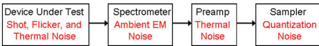
Fig. 1. Signal path in our EDMR spectrometer illustrating the types of introduced as well as the sources.
