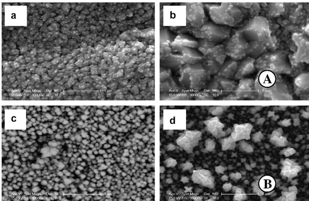
Fig. 1. Surface morphology and chemical composition variations with current density and plating time ( $\text{A}/\text{dm}^2\text{-s}$ ); (a) 1–30, (b) 1–60, (c) 1.5–30 and (d) 1.5–60.
