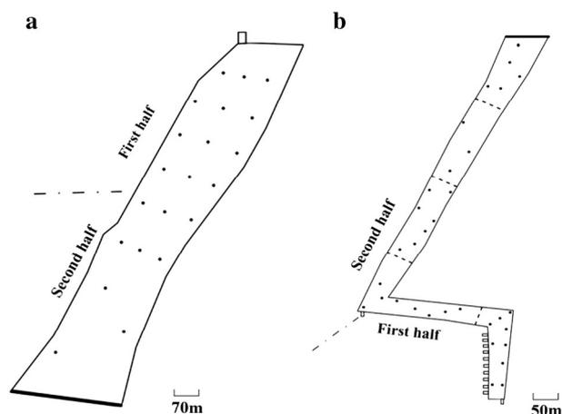
Fig. 1. The schematic diagrams of the W-CW (a) and Q-CW (b). Circles represent sampling points (21 points in W-CW while 31 points in Q-CW), and squares stand for the inlets. The bold lines instead for the outlet and the dashed lines instead for the overflow weir.
