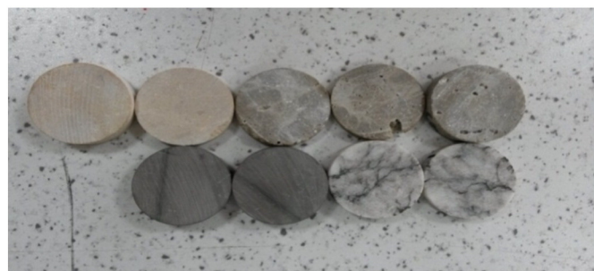
Fig. 1. Samples of rock slices with 0.5 cm thickness and 3.79 cm diameter which has been cut from the selected core samples.
