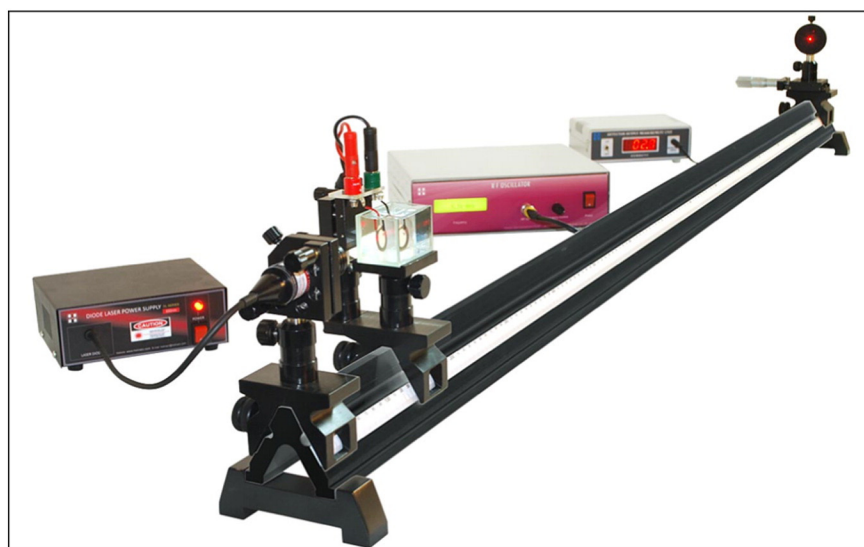
Fig. 1. Experimental setup of ultrasonic-laser diffraction.
