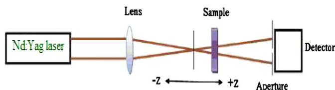
Fig. 1. Schematic diagram of the experimental arrangement for close aperture z-scan setup.
