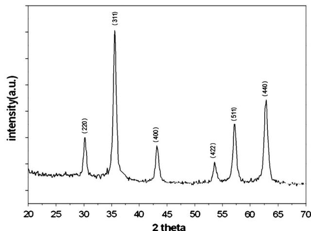
Fig. 2. XRD pattern of synthesized Fe<sub>3</sub>O<sub>4</sub> nanoparticles matching to the standard JCPDS no. [03-065-3107].
