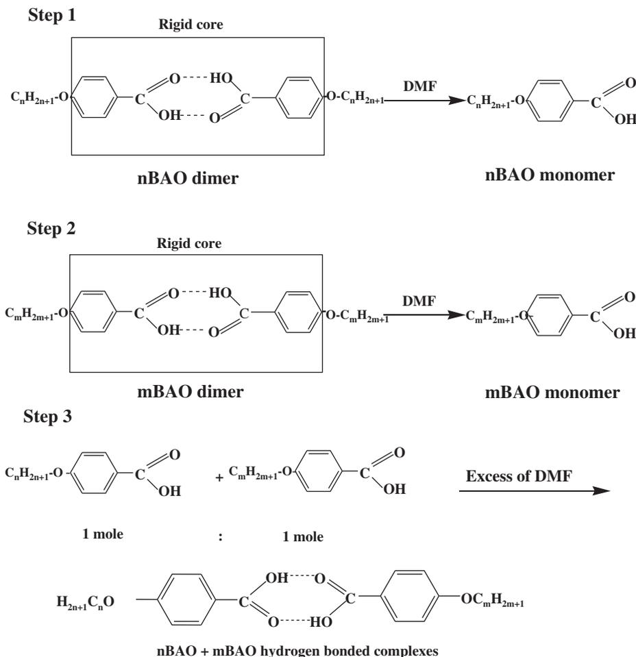
Scheme 1. Scheme representing the formation of 10BAO + mBAO hydrogen bonded series.
