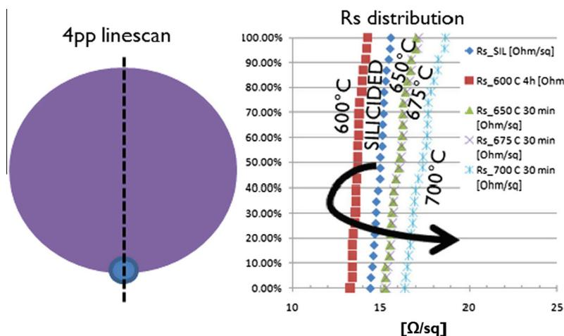
Fig. 1. (left) Sketch of line scan used for the 4-point sheet resistance measurement. (right) Evolution of the cumulative distribution for sheet resistance with the additional thermal treatments. In the presented case, the evolution of both median and spread with the temperature of the anneals is clearly visible.
