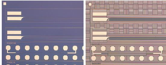
Fig. 2. Different layouts used within the CMP investigations.
