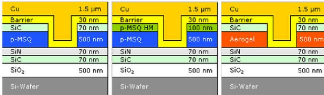
Fig. 1. Schematics of single damascene interconnect based on p-MSQ and SiO<sub>2</sub>-aerogel as used in the CMP experiments.
