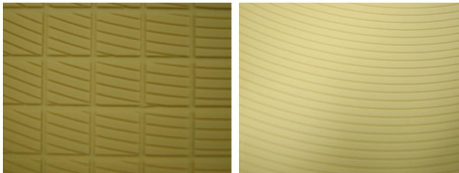
Fig. 4. Groove layout of CUP4410™ (left) and IC1010™ (right) polish pads.
