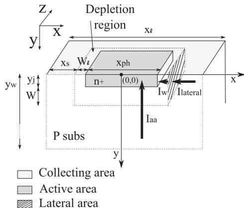
Fig. 1. Cross section of the photodiode 3D structure.
