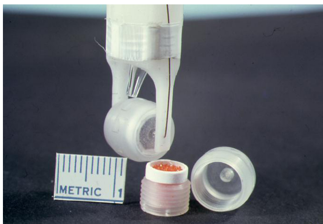
Fig. 1. Spinning system for the original CPMAS experiment [1]. The photograph provided courtesy of Prof. Jacob Schaefer at the Washington University in St. Louis. “The rotor was suspended from two phosphor-bronze wires held to the “stator” by teflon tape. A pipette brought the drive air in. A rotor would only last through 2 or 3 stop–start cycles. It took Ed (Stejskal) a day to make a rotor,” according to a note from Prof. Schaefer.
