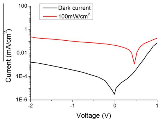
**Fig. 2.** Current–voltage characteristics of the PCPDTBT:ZnO photodiode under dark and with incident power of  $100 \text{ mW/cm}^2$ .
