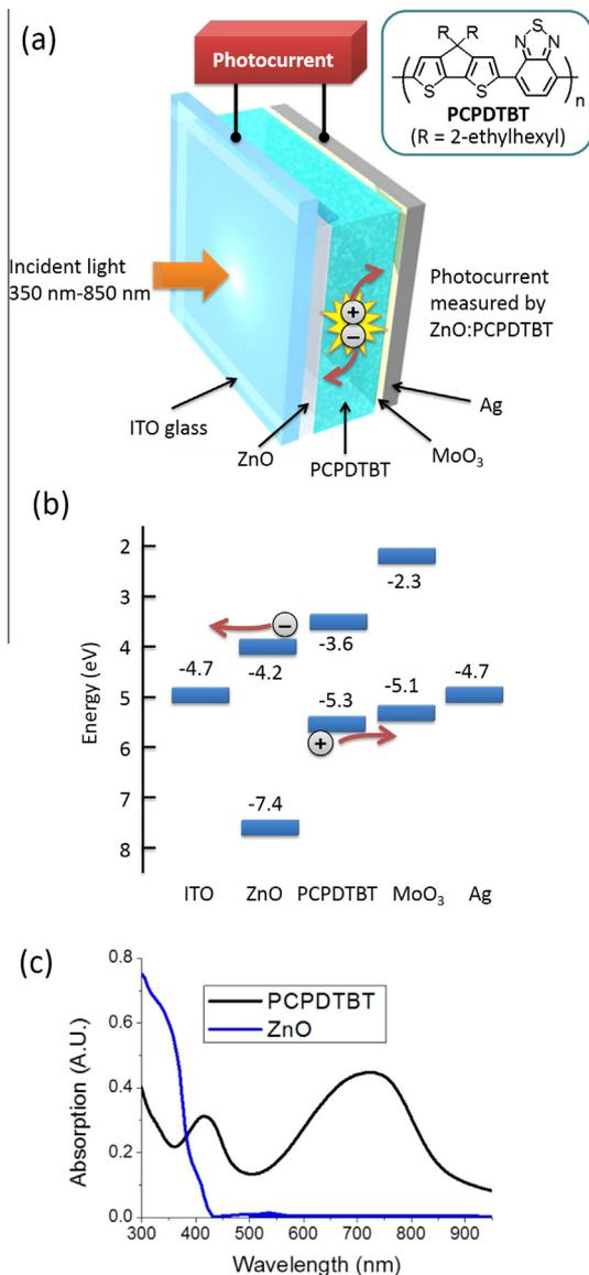
**Fig. 1.** (a) Schematic of the photodiode and (b) ideal flat band energy diagram for a PCPDTBT:ZnO photodiode (assuming ZnO  $E_v = -7.4$  eV,  $E_c = -4.2$  eV from [10]). Light is incident from the ITO side of the device. Other workfunction data is obtained from [14]. (c) Absorption profile of PCPDTBT and ZnO layers.
