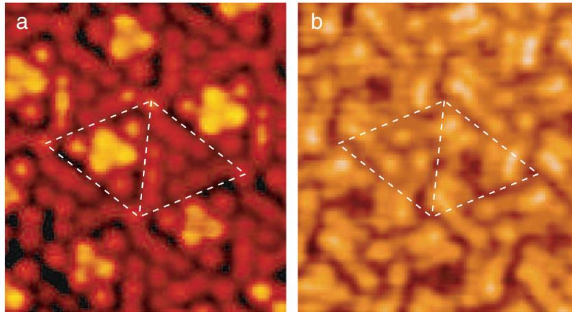
**Fig. 1.** (a) Empty-state (+1.8 V) and (b) filled-state (-1.8 V) STM images of the Si(111) $\sqrt{31} \times \sqrt{31}$ -In reconstruction. Unit cell with two triangular subunits is outlined by the dotted line.
