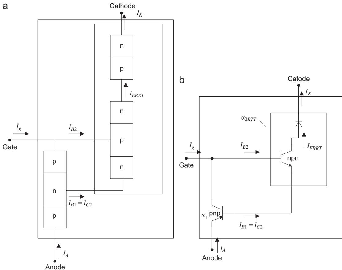
Fig. 1. Currents in a two-transistor model for the RT-SCR: (a) the semiconductor regions, (b) circuit symbols.
