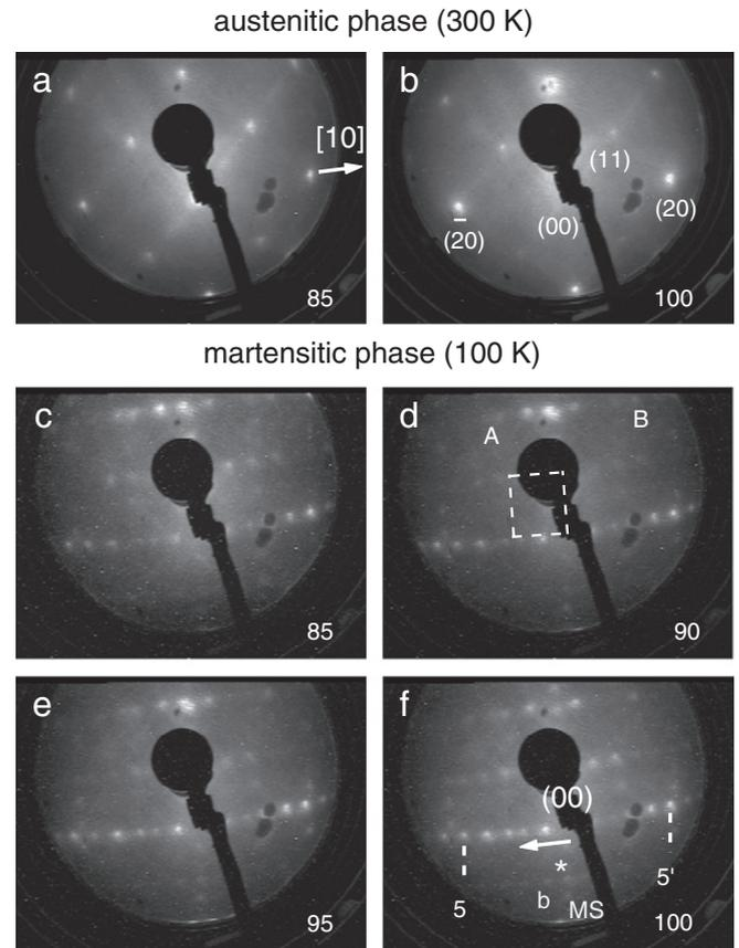
**Fig. 1.** Low energy electron diffraction (LEED) patterns of  $\text{Ni}_2\text{MnGa}(100)$  in (a–b) the austenite phase at room temperature and in (c–f) the martensite phase at 100 K. The electron beam energies ( $E_p$ ) in eV are shown in the bottom right corners. The first Brillouin zone (white dashed square) and the direction AB along [10] outside first Brillouin zone are shown in (d). In (f), dashed lines indicate the 5 and 5' spots and the white arrow represents  $b_{MS}^*$ .
