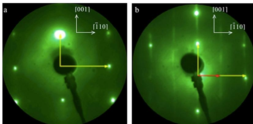
Fig. 1. LEED patterns recorded at 44 eV primary energy: (a) ( $1 \times 1$ ) of a clean Ag(1 1 0) substrate; (b) ( $2 \times n$ ) superstructure of SiNWs adsorbed onto Ag(1 1 0) at RT.
