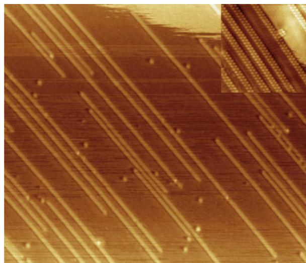
Fig. 2.  $70 \text{ nm} \times 80 \text{ nm}$  STM image of SiNWs adsorbed onto Ag(1 1 0) at RT,  $I_t = 0.47 \text{ nA}$ ,  $V_{\text{bias}} = -600 \text{ mV}$ , filled states. The top-right inset corresponds to a zoom-in of  $10 \text{ nm} \times 10 \text{ nm}$ ,  $I_t = 0.32 \text{ nA}$ ,  $V_{\text{bias}} = -20 \text{ mV}$ , filled states.
