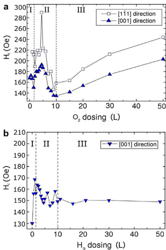
Fig. 1. Evolution of the coercive field as a function of (a) O<sub>2</sub> and (b) H<sub>2</sub> dosage on the clean Co/Cu{110} surface.
