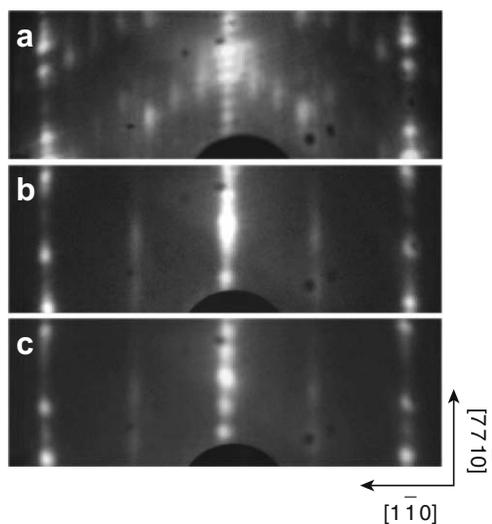
**Fig. 1.** LEED patterns of (a) the clean surface and (b) and (c) the Ag-induced  $\times 2$ -structured surface on Si(557). The sample was prepared at 500 and  $610^\circ\text{C}$  during Ag deposition on (b) and (c), respectively. The incident electron energy was 40 eV.
