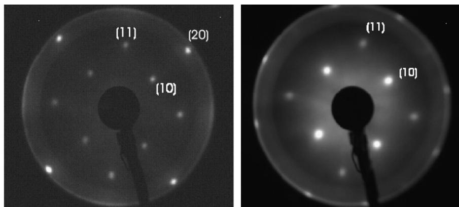
Fig. 1. Left: LEED pattern of the RbBr(100) surface at a primary electron energy of 86 eV and a temperature of 156 K. Right: LEED pattern of the RbI(100) surface at 68 eV and 183 K.
