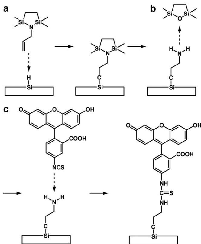
Fig. 1. Schematic view of immobilization of FITC on an aminopropyl monolayer: (a) thermal reaction between protected-allylamine and H-Si, (b) hydrolysis of the protecting group in an acidic solution, and (c) anchoring of FITC to the aminopropyl monolayer.
