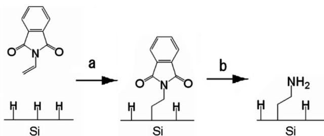
Fig. 2. Preparation of an amino-terminated monolayer through the hydrolysis of phthalimide: (a) reaction between vinylphthalimide and H-Si to form a phthalimide monolayer and (b) hydrolysis of phthalimide to form an amino-terminated monolayer.
