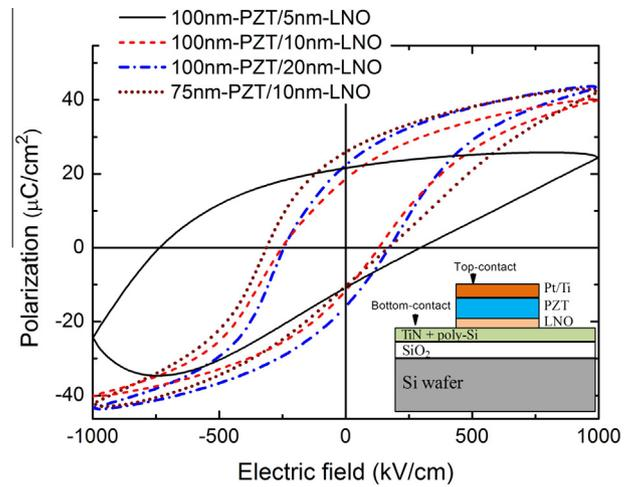
**Fig. 2.** Thickness dependence of polarization hysteresis (P–E) loops. The P–E loops were performed at an applied ac electric field of ±1000 kV/cm and 1 kHz frequency. The inset shows the schematic cross section of the test structure.
