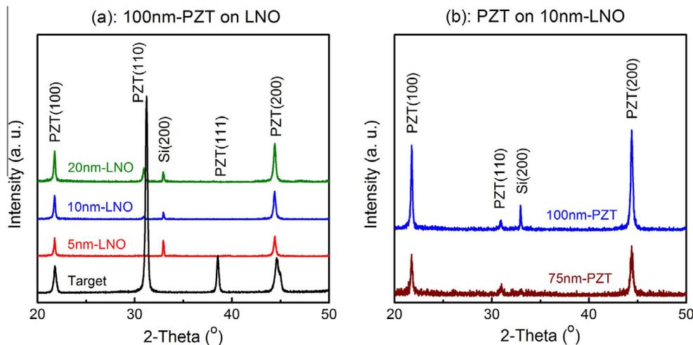
**Fig. 1.** XRD graphs of (a) a 100 nm-thick PZT film on different LNO layer thicknesses and (b) a 75 nm and a 100 nm PZT film on a 10 nm-thick LNO layer.
