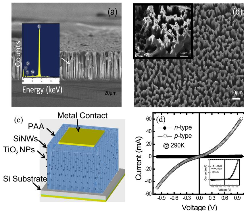
**Fig. 1.** (a) Cross-sectional SEM image of SiNWs/PAA/TiO<sub>2</sub> NPs composite device with EDS spectra (inset). (b) Planer SEM image of composite device and inset shows planer SEM image after plasma etching (similar images were seen in both *n* and *p*-SPT composite devices). (c) Schematic diagram of fabricated composite device. (d) Comparison of IV characteristics at 290 K and 77 K for *n*-SPT and *p*-SPT composite devices.
