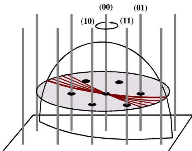
Fig. 1. Geometry of a RHEED azimuthal scan.
