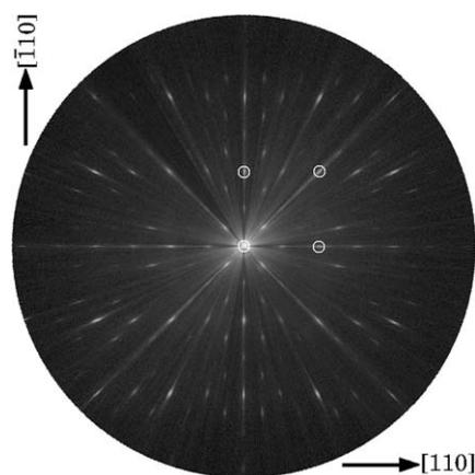
Fig. 2. Azimuthal RHEED scan of the GaAs  $c(4 \times 4)$  surface immediately before MnAs deposition. The corners of the surface unit cell are marked by circles.
