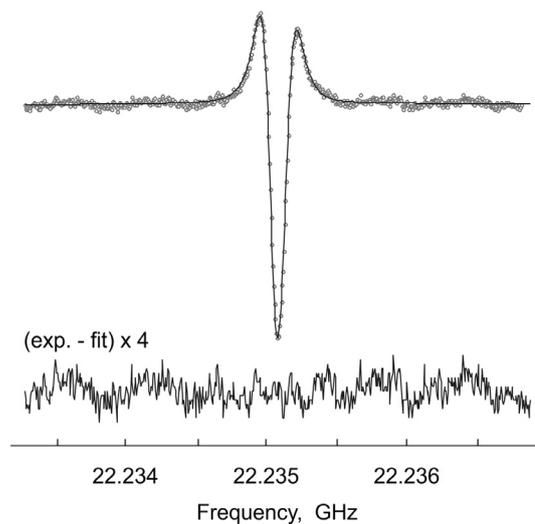
**Fig. 2.** Line recording in pure water vapor at 4.75 mTorr obtained with video spectrometer using FM regime (upper trace) and the result of model function fitting to the observed spectrum (lower trace).
