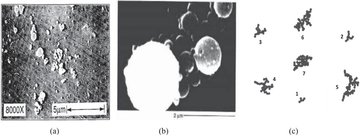
Fig. 1. The pictures of alumina particles in the plume. (a) The typical scanning electron microscope photo of alumina particles in the plume [6]; (b) Alumina particles produced in a rocket motor [3]; (c) Some examples of the alumina fractal aggregates are simulated using the DLA algorithm. The parameters of these particles are:  $k_f = 1.2$  and  $a = 100$  nm. (1)-(4)  $N_s = 5, 10, 20$  and  $35, D_f = 1.82$ ; (5)-(7)  $N_s = 50, D_f = 1.62, 1.82$  and  $2.11$ .
