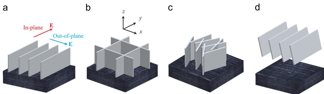
**Fig. 1.** A sketch of the different graphitic petals we considered: (a) grating, (b) cavity, (c) random cavity, and (d) oblique gratings. For vertical grating and oblique grating, in-plane polarization is defined as the electric field parallel to the graphitic petal and out-of-plane polarization is defined as the electric field perpendicular to the graphitic petal.
