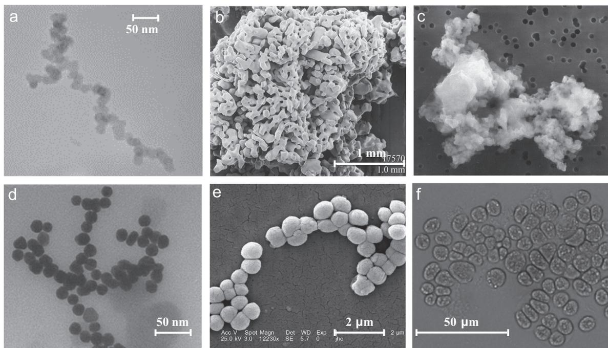
**Fig. 1.** Micrographs of fractal aggregates of (a) soot [9], (b) snow [10], (c) cosmic dust [11], (d) gold nanoparticles [12], (e) the bacteria *M. luteus* [13], and (f) colony of the microalgae *B. braunii*.
