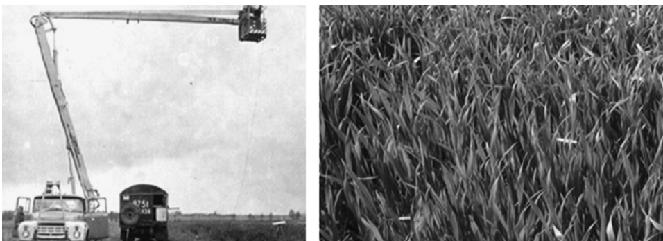
Fig. 1. Remote sensing measurements of the reflection factor of plant canopies using a spectrophotometer installed on the elevated work platform.
