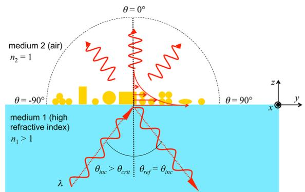
Fig. 1. Schematic representation of the characterization framework: particles on the substrate are illuminated by an evanescent wave generated by TIR of an external radiation beam.
