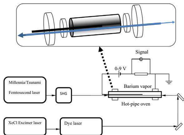
Fig. 1. The experimental setup with thermionic diode detection system.
