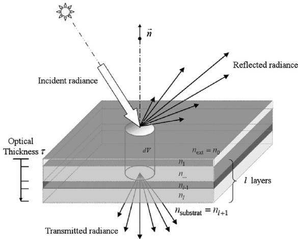
Fig. 1. Schematic of a generic dense scattering medium modeled as semi-infinite multiple layers.
