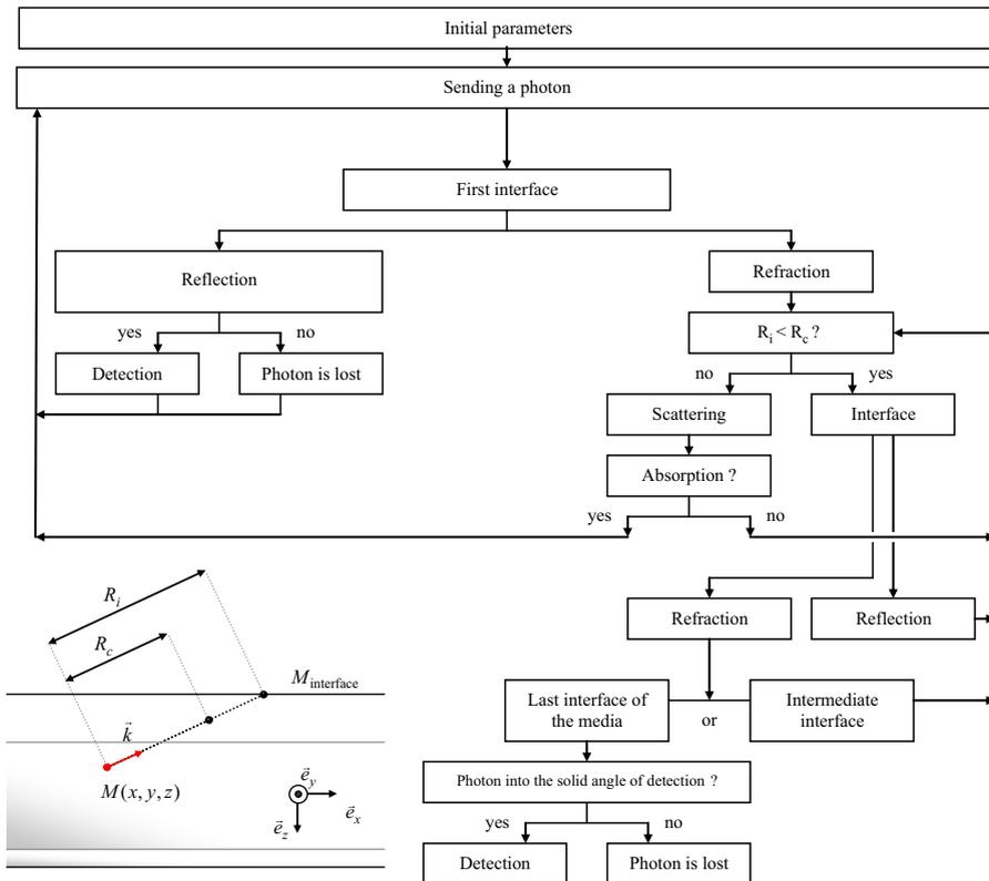
Fig. 2. General Monte Carlo scheme of a multi-layered media. Reflection and refraction are considered at each interface. Polarized scattering events include the possibility of light absorption by the scatter. The incident Stokes vector is modified by the  $4 \times 4$  Mueller matrix.
