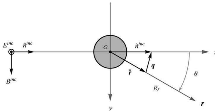
**Fig. 1.** Scattering arrangement consisting of a spherical particle illuminated by a linearly polarized plane wave. The observation point  $\mathbf{r}$  is confined to the  $y$ - $z$  plane at a fixed radial distance  $R_l$  from the particle. The polarization of the incident wave is normal to  $y$ - $z$  plane. Also indicated is the direction of the scattering wave vector  $\mathbf{q}$ , Eq. (2).
