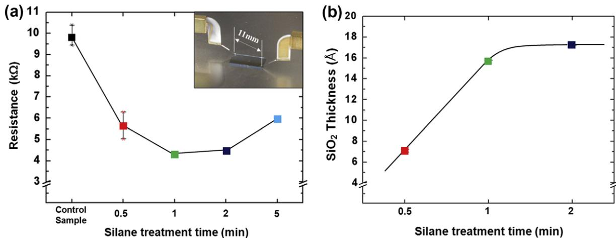
**Fig. 2.** (a) The electrical resistance of epitaxially grown graphene samples after a silane pre-treatment with various silane treatment times. The resistance was measured by probing two locations of the graphene layers with a fixed distance of 11 mm (see the inset image). (b) The thickness of  $\text{SiO}_2$  grown by sacrificial oxidation, on the surface of silane-treated SiC wafers with different silane treatment times.
