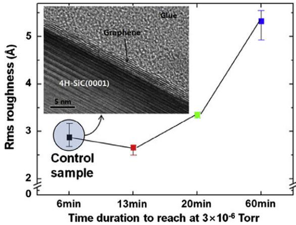
**Fig. 1.** The rms roughness of graphene layers with respect to the pumping down time to reach a vacuum level of  $3 \times 10^{-6}$  Torr. Graphitization was done at  $1430^\circ$  for 10 min. Inset: TEM image of a graphene layer when the pumping down time is 6 min.
