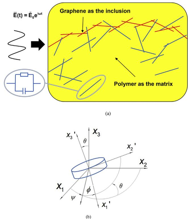
Fig. 1. (a) Schematic of the graphene-polymer nanocomposites subjected to AC electrical loading, (b) schematic of Euler angles describing the orientation of graphene filler with respect to the Cartesian coordinate. (A colour version of this figure can be viewed online.)
