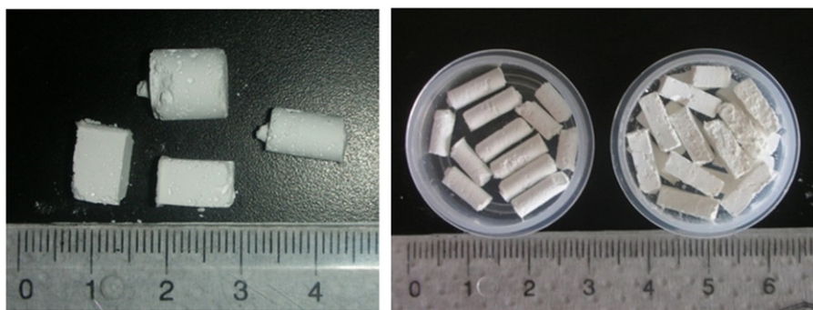
Fig. 1. Hydroxyapatite objects molded in different sizes and shapes by the Modified GelCasting Process (scale in cm).
