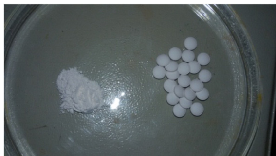
Fig. 1. Formation of tablets from the powdered composite of EC-MgHPO 4 .
