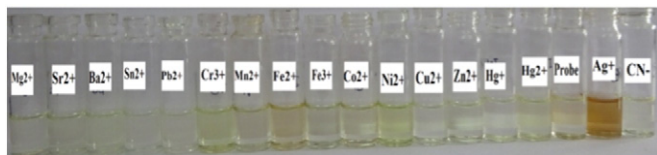
Fig. 1. Naked eye detection of \text{Ag}^+ and \text{CN}^- with probe.
