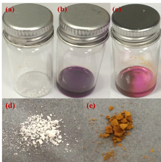
Fig. 1. Photo images of ZIF-8 powder and iodine solution. (a) and (d) ZIF-8 before iodine adsorption; (b) iodine dissolved in n-heptane, (c) iodine solution after ZIF-8 adsorption; (e) ZIF-8 powder after iodine adsorption.
