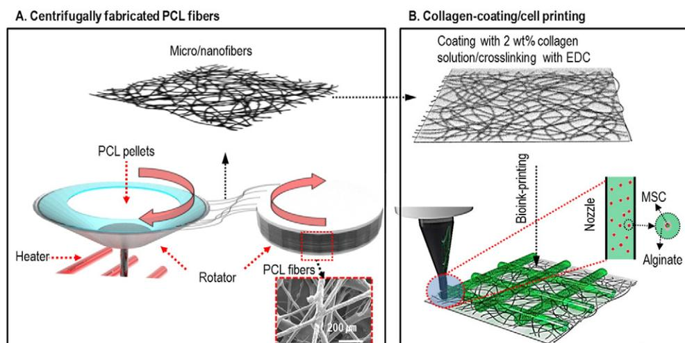
**Fig. 1.** Schematic diagram of the fabrication procedure for the MSCs-laden fibrous structure. (A) Centrifugal melt-spinning for PCL fibers. (B) Collagen-coating/cell-printing process for MSCs-laden fibrous structure (PCAMSC).
