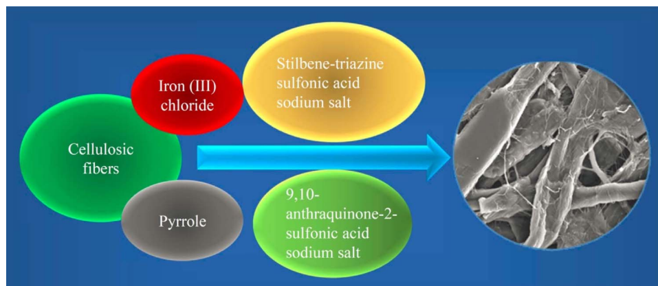
Fig. 2. Schematic of converting cellulosic fibers into polypyrrole-engineered fiber product (i.e., paper-based product) involving the use of stilbene-triazine sulfonic acid sodium salts.
