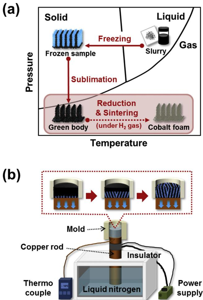
Fig. 1. (a) Schematic phase diagram of water illustrating phase changes in the liquid aqueous slurry during the ice-templating and sintering processes and (b) schematic illustration of ice-templating device and directional slurry freezing process.
