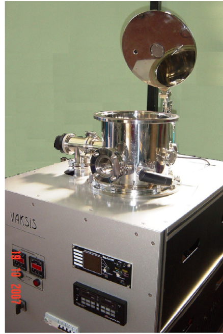
THERMAL EVAPORATION SYSTEM
