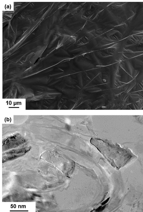
Fig. 1. (a) SEM image showing a network of long nanotube clusters well meshed in Al matrix post solidification. (b) Low magnification TEM image showing long and intact BNNTs in cast Al-BNNT composite.
